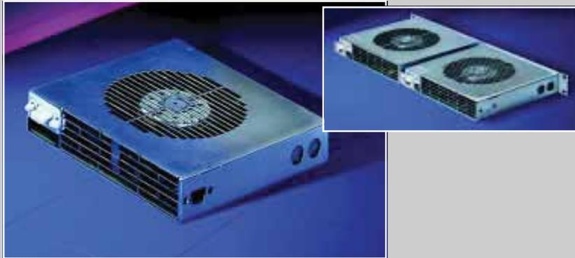
The powerful RiCool blower assembly is specially designed to provide effective cooling in densely packed systems where the average board has a heat loss of above 30 Watts at 21 slots and performs well at an average heat loss at 70W per PCB (at 21 slots). Low noise (48dBa at <sup>3</sup>/<sub>4</sub> speed and a life of approx. 60,000 hrs at 40°C) makes this blower the ideal solution for today's systems.
