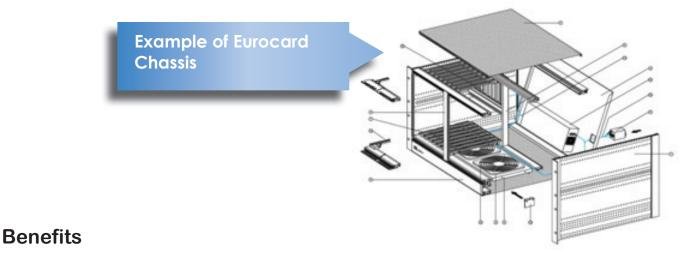
The benefits of Eurocard is the ability to utilize a common PCB and subrack framework to base your design around. Perhaps the largest benefit is using a modular, standardized format that entire industries are familiar with – creating a standard product ecosystem from which to start. The standardization significantly reduces development costs, reduces time to market, and allows a wide range of potential suppliers to offer to standard or "modified-standard" solutions.
