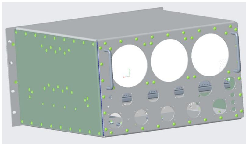
Drawing of Example #2 (Front to Rear Airflow, Recessed, SOSA Aligned)
